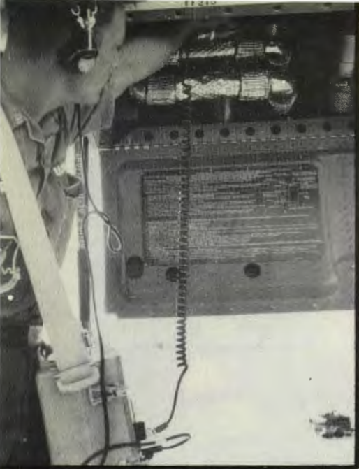
Ultrasonic leak detector can pinpoint liquid and gaseous leaks in a hurry. An F-105 oxygen system and a C-130's maze of plumbing get a close going over.
