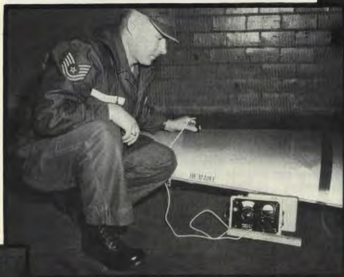
A conductivity meter probes a T-39 nacelle for cracks.
