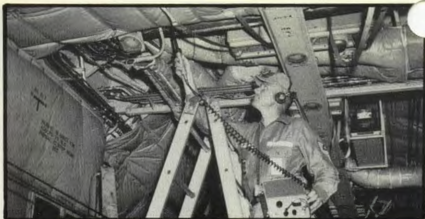
Ultrasonic leak detector can pinpoint liquid and gaseous leaks in a hurry. An F-105 oxygen system and a C-130's maze of plumbing get a close going over.
